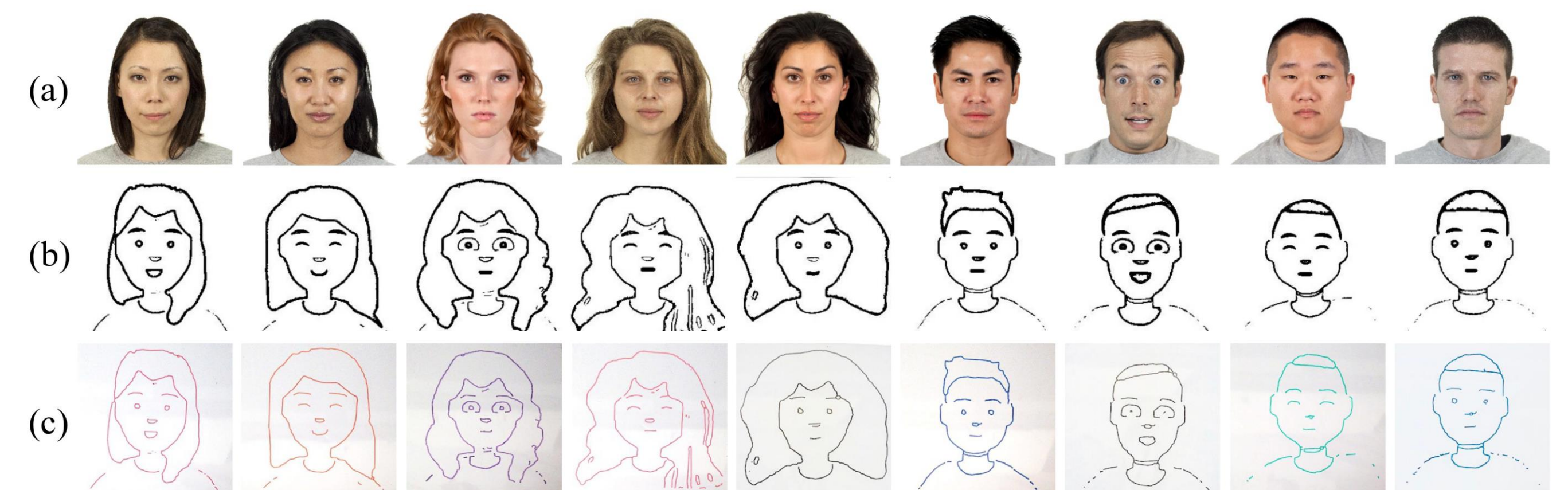
Fig. 8 (a) Face images and (c) whiteboard drawings generated from (a) face image using the integrated RoboCoDraw System
